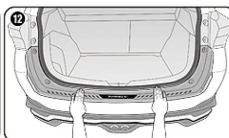
Press the rear bumper guard firmly to vehicle.
