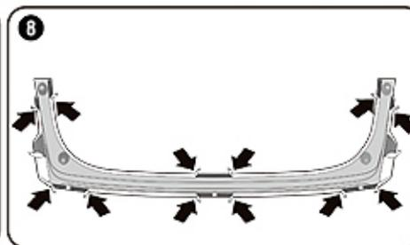
Peel off a small parts of double sided tape a bit as shown.
