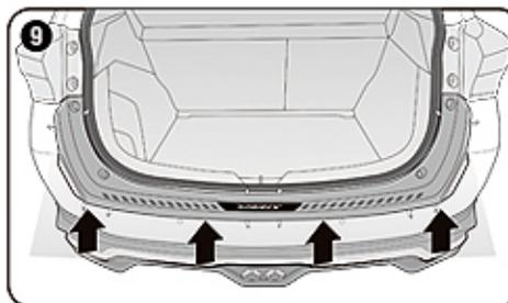
Mounting rear bumper guard on position as shown.
