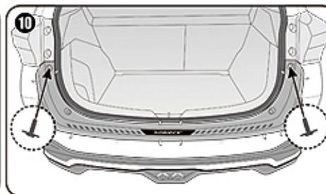
Reassemble screw to original position as shown.
