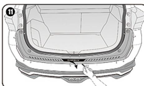
Peel off the rest of double sided tape as shown.
