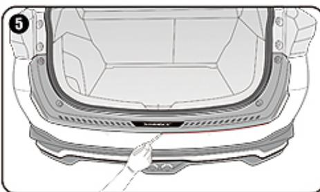
Marking the position with crayon as a guide for double sided tape.
