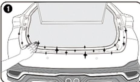
Wipe installation area clean with alcohol for better adhesion.
